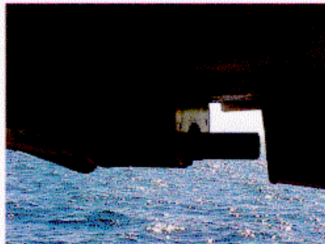
Figure 2 - Reson SeaBat 8101 hull-mounted in keel cut-out of Launch 1005.
