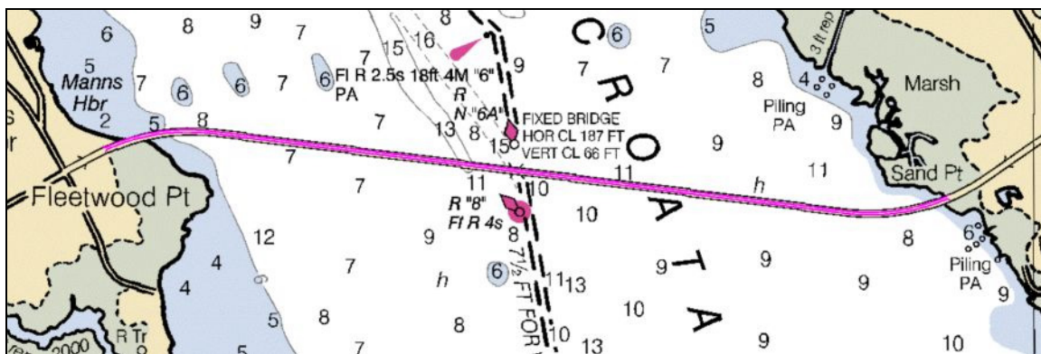
Surveyed position of newly constructed Bridge (magenta) Chart 12204 35 th Ed., in background
