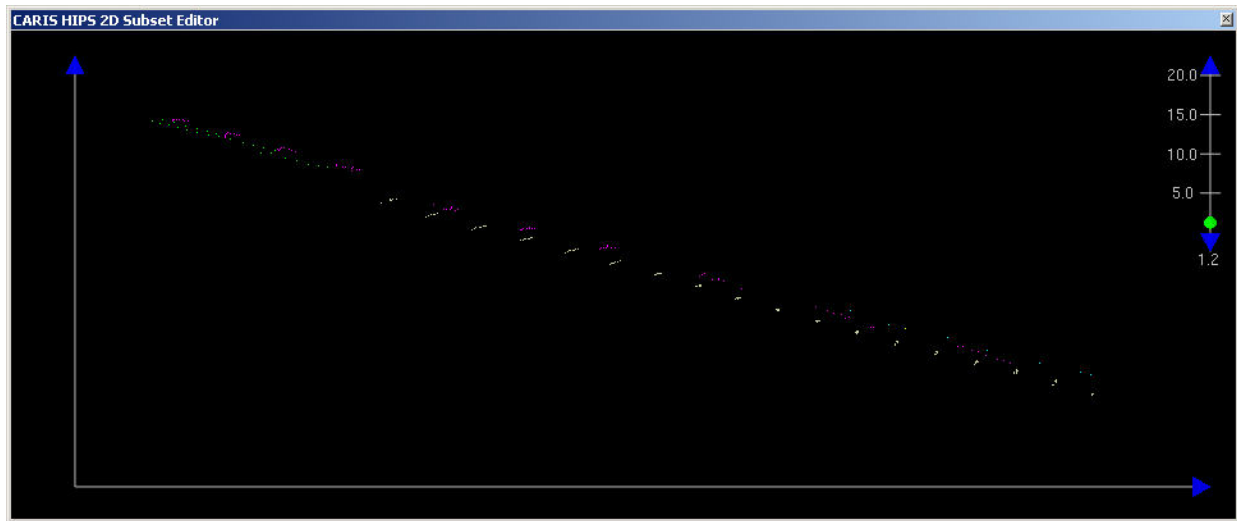
Figure 3. Line offset in outer beams of survey H11124 shown in Caris HIPS 5.4 Subset Editor.
