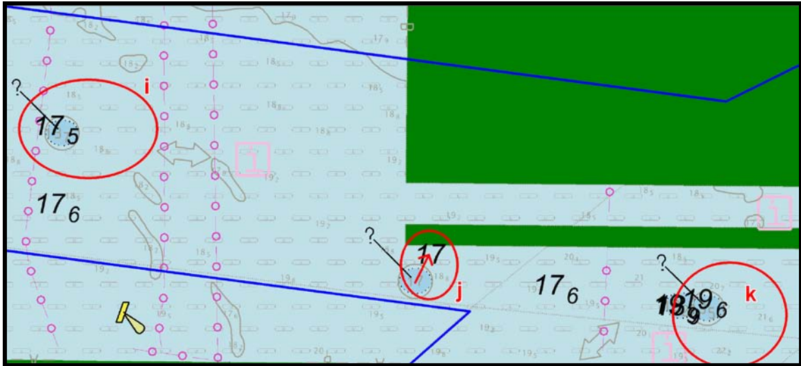
Figure 21—Overview of survey area H-11547, covered by ENC US4AL11M, 13 th Edition, showing three of the four features identified in the 2006 survey that differ significantly from the corresponding charted features. The features are circled in red and assigned a letter designator that corresponds to the details in Tables 6-7. All soundings are in meters.
