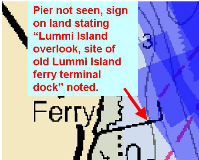
24. Site of old Ferry Terminal partially covered with MBES and SSS in blue overlaid on chart 18430.
