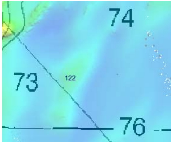
Figure 7. The least depth of 122 meters (66.5 fm) over a new shoal is shown in the center of a triangle of charted (16553) depths of 73, 74 and 76 fm. A 5-m CUBE Surface colored by depth is overlain on chart 16553.
