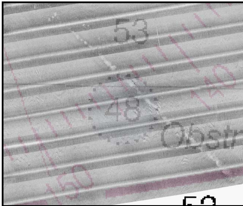
Figure 10 -Side Scan Mosaic of a charted obstruction near AWOIS 8708 overlain on Chart 11376, 51 st Edition. The hydrographer recommends removing the obstruction from the chart.
