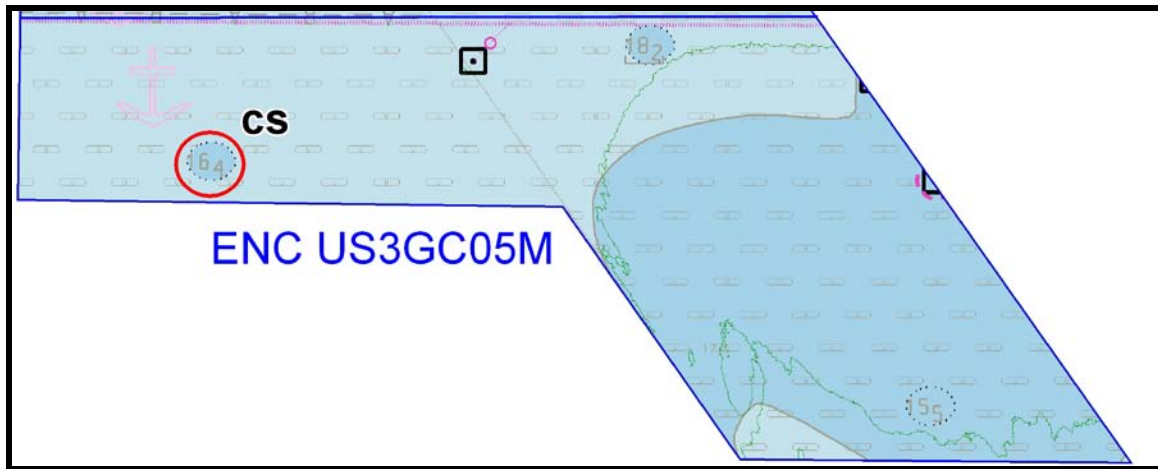
Figure 30 - Overview of survey area H-11583, covered by ENC US3GC05M, 8 th Edition, where features identified in the 2006 survey are significantly shoaler and/ or horizontally offset from the corresponding charted features.
