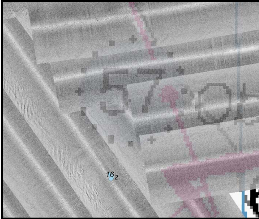
Figure 11 –Side Scan Mosaic of a charted obstruction near AWOIS 8709 overlain on Chart 11376, 51 st Edition. The hydrographer recommends moving the charted obstruction south to the location of the contact (blue circle).
