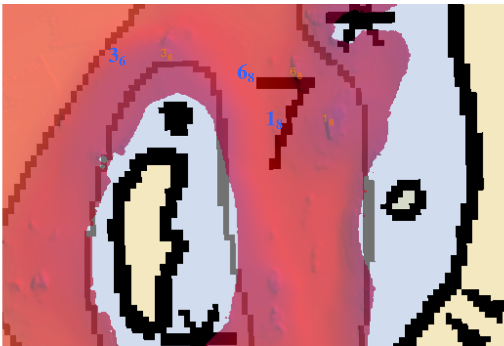
Figure 17. A 2-m CUBE surface colored by depth is overlaid over chart 16708 in Caris HIPS 6.1. Soundings were designated over 2 new shoals surveyed in the vicinity of a charted 7-fm (12.9 m) sounding, and are displayed in blue with depth in meters.
