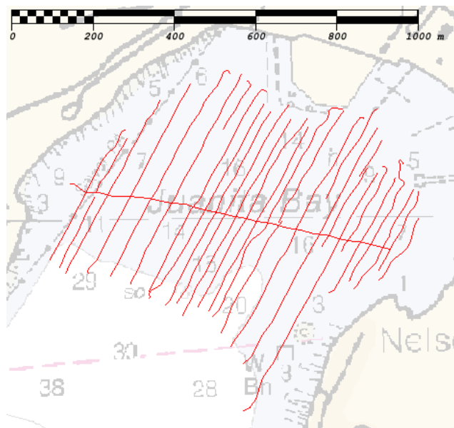
Figure 8: Ceeducer line data in Juanita Bay flagged as 'Reject Line' in Caris HIPS and SIPS.
