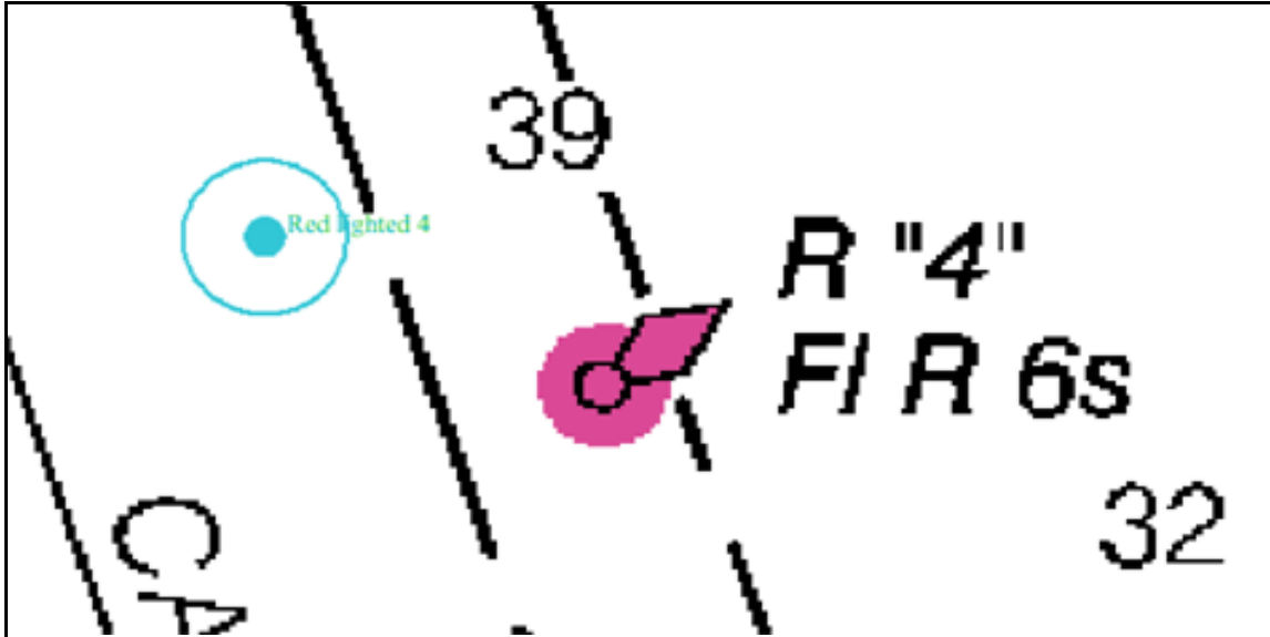
Figure 31. The detached position (cyan) is shown in reference to Buoy 4 on RNC 11384. The DP was obtained prior to Buoy 4 being reported as Off Station in LNM 50/09. The USCG has since reset the buoy to its charted position.
