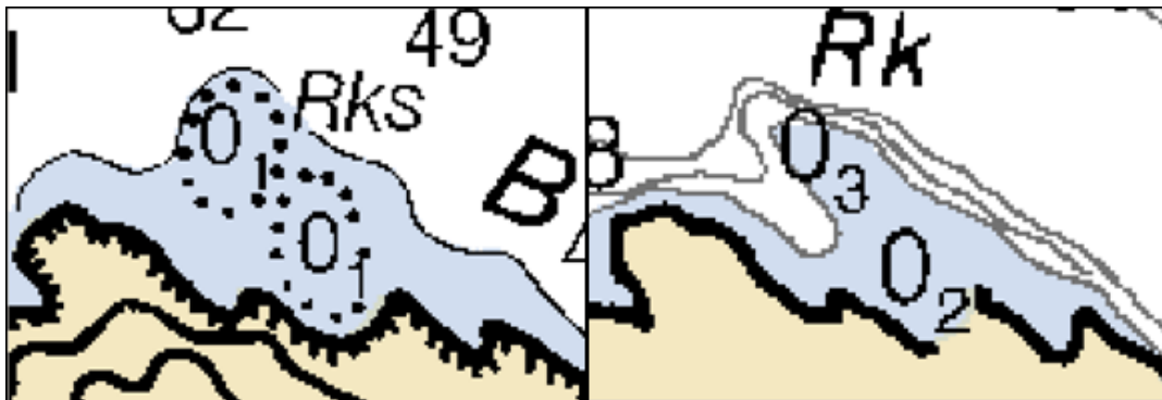
Figure 10: Discrepancy between Chart 16645 (left) and Chart 16647 (right) in approximate position 59^{\circ}26'11''N 151^{\circ}22'13''W . Survey found least depth of 0-fathoms 1.6-feet on the offshore feature and 0-fathoms 0-feet on the inshore feature.
