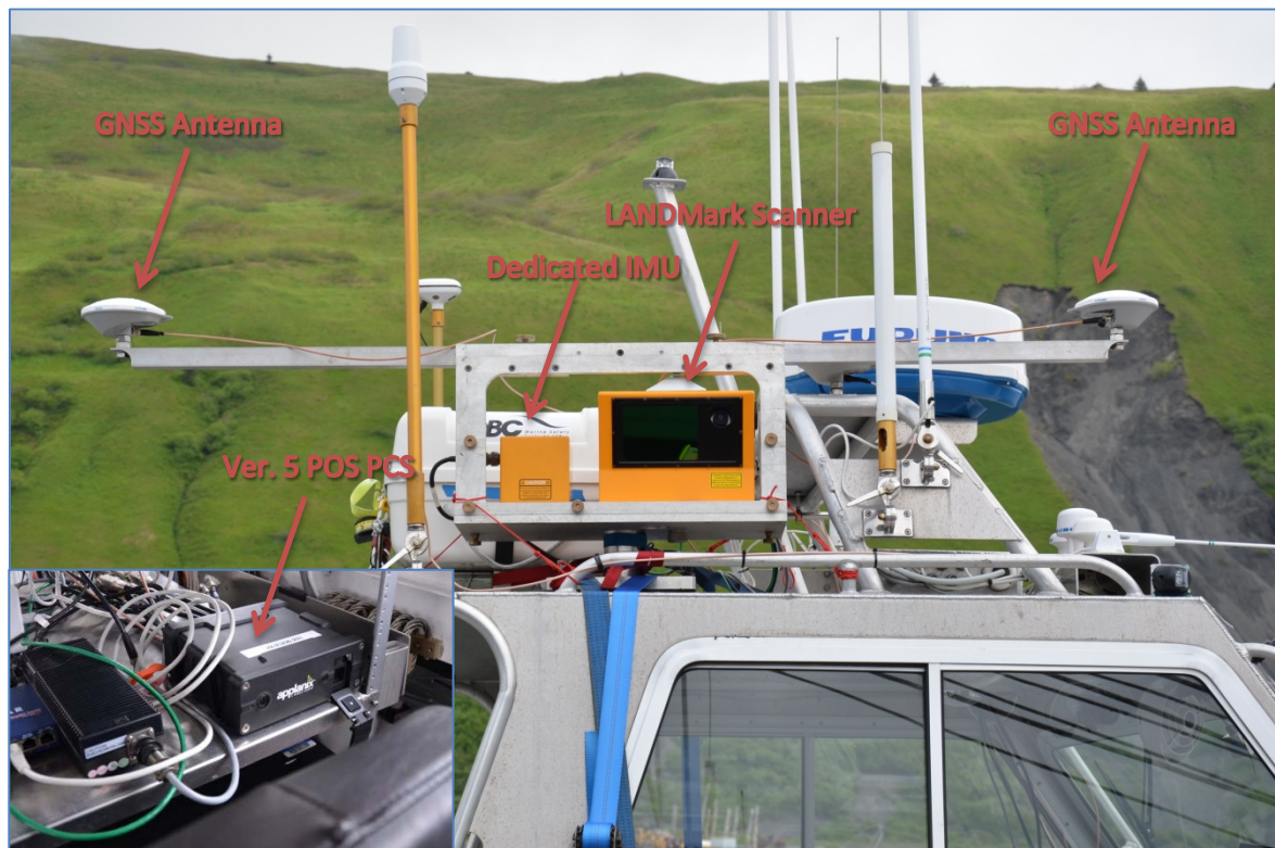
Figure 1. LANDMark Laser installed on 2808
