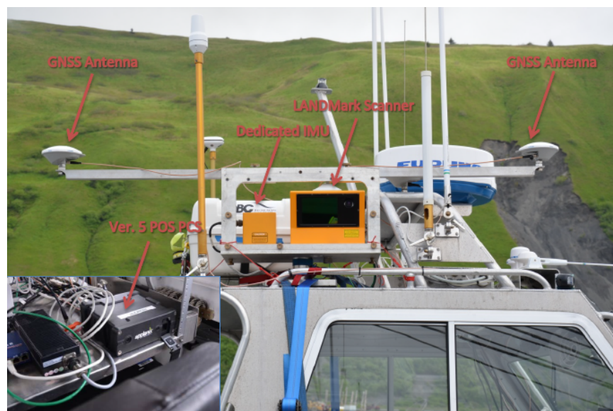
Figure 2: Launch 2808 With Mounted LANDMark Marine Laser Scanner
