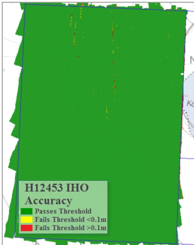
Figure 14: H12453 met IHO accuracy standards for 99% of the data. Green passed the IHO threshold. Yellow failed the threshold by less then 0.1 meters. Red failed the threshold by greater than 0.1 meters.
