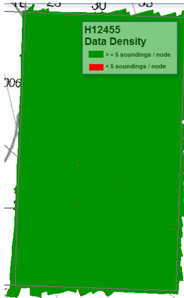
Figure 2: H12455 data density. Areas in green meet the threshold of 5 soundings per node; red areas have a data density less than 5 soundings per node.
