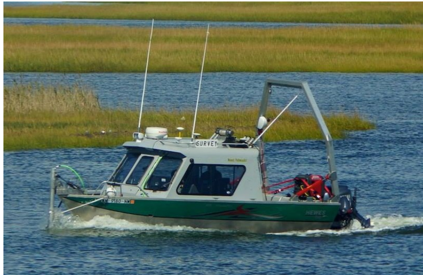
Figure 7: M/V Nooit Volmaakt from the port side. The pole mount on the bow for the Edge Tech SSS can be seen.
