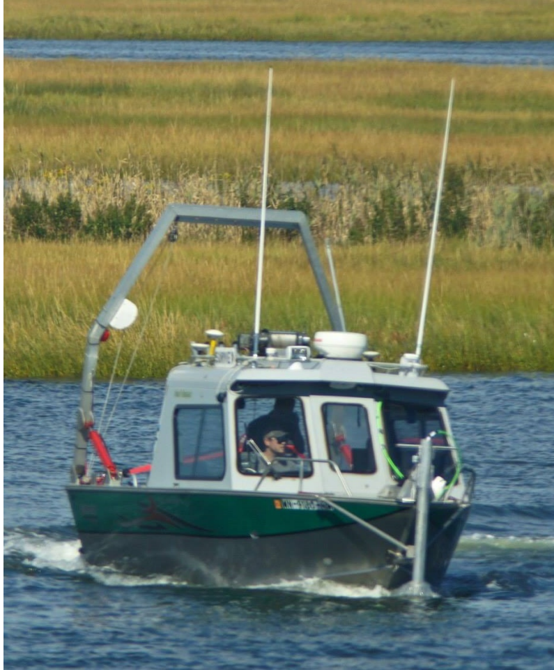
Figure 8: M/V Nooit Volmaakt from the starboard bow. The pole mount on the bow for the Edge Tech SSS can be seen.
