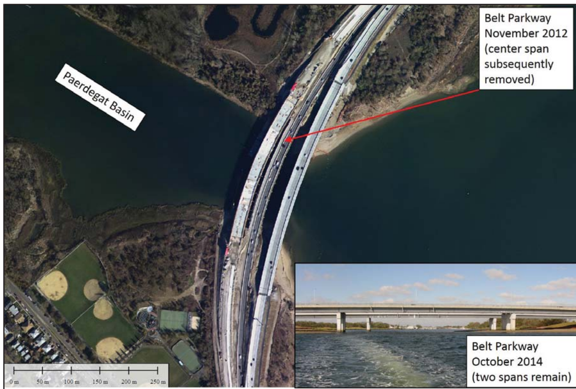
Figure 43: Aerial imagery captured the change in the Paerdegat Basin Bridge from one span to two spans during Belt Parkway construction.
