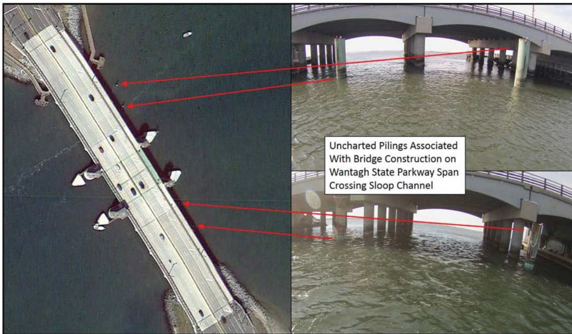
Figure 46: Aerial imagery and photographs acquired during survey acquisition show the uncharted pilings associated with bridge construction of the Wantagh State Parkway span crossing Sloop Channel.
