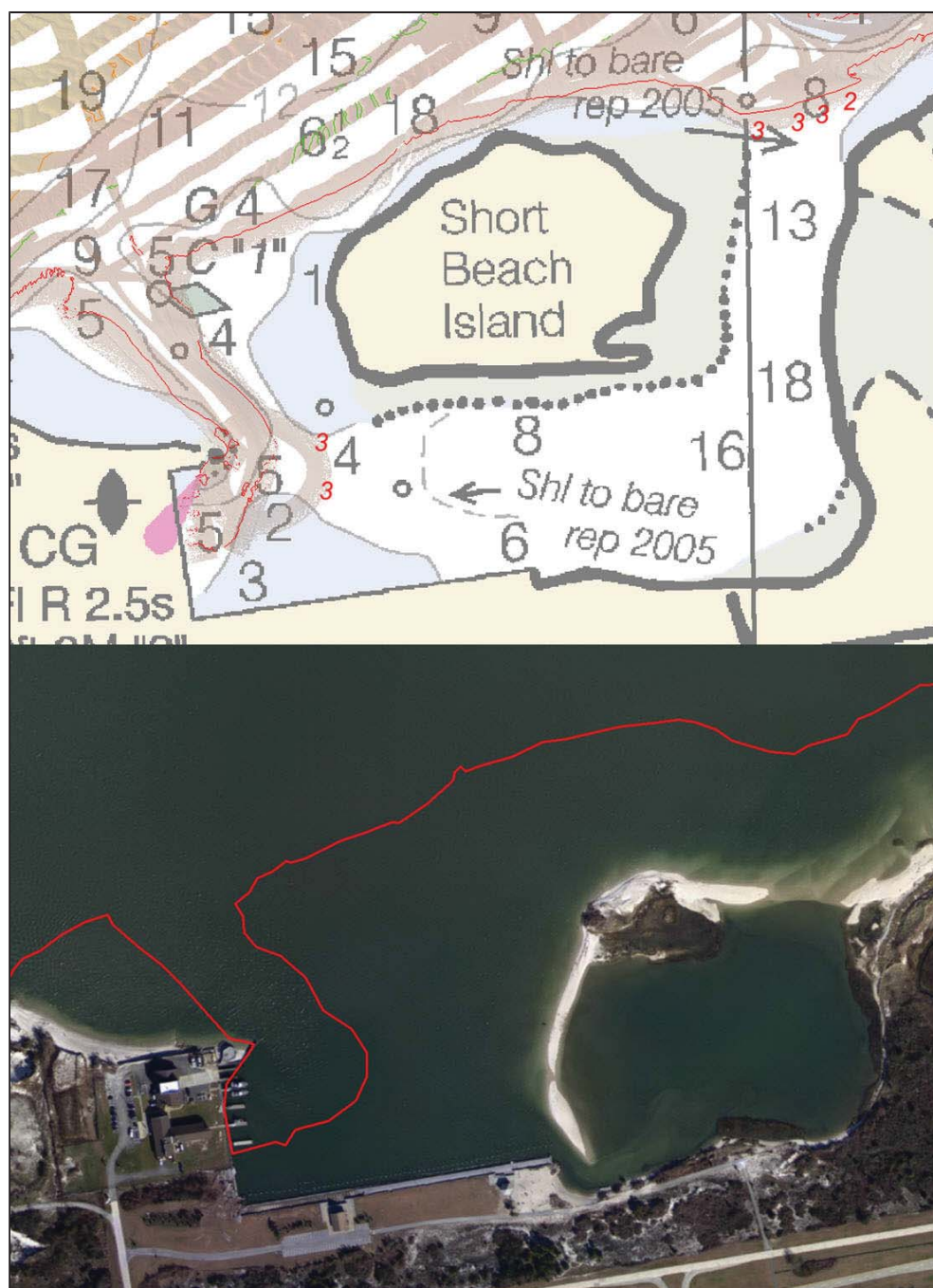
Figure 39: In the top image, contours generated from the H12607 MBES data (6' in red, 12' in green, and 18' in orange) are shown in reference to Short Beach Island. Representative soundings of the shoaling surrounding the island are highlighted in red with a CUBE surface overlaid on RNC 12352 in the background. In the image on the bottom, NGS post-Sandy imagery of Short Beach Island is shown with the H12607 survey outline highlighted in red.
