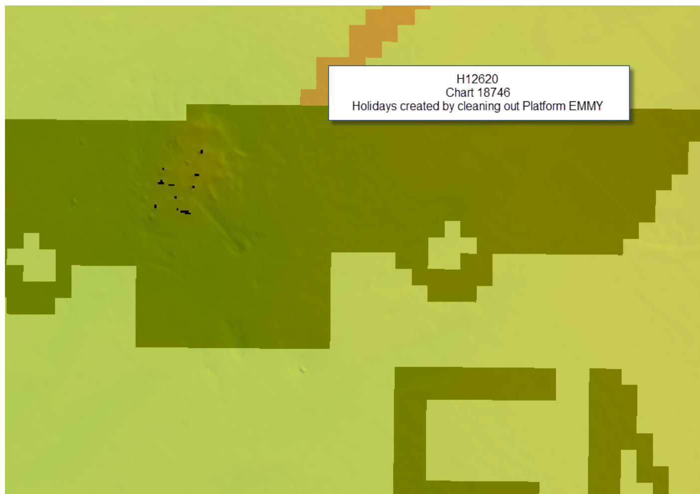
Figure 13: H12620 Holidays due to cleaning of Platform EMMY (chart 18746) from the HIPS Surface.
