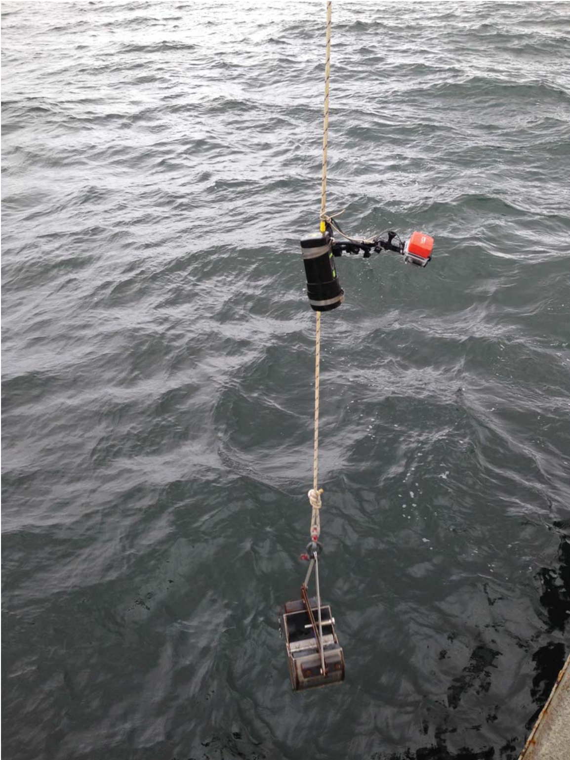
Figure 26: Bottom sampler used for H12696 with attached video camera
