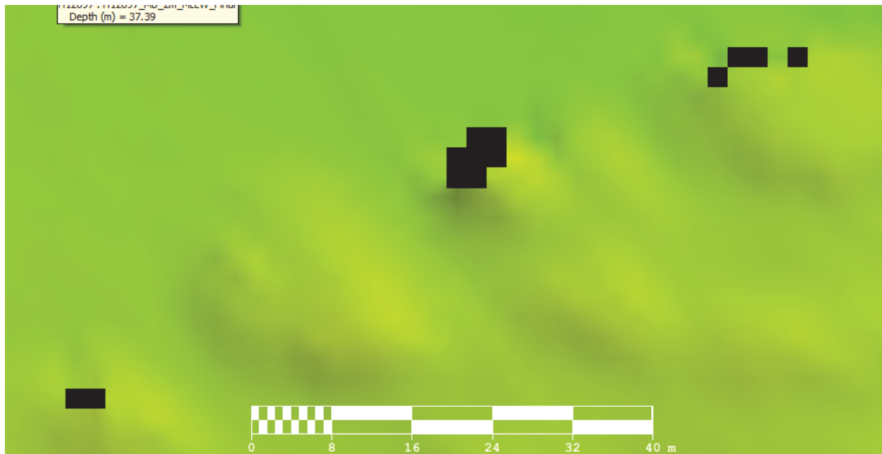
Figure 17: Example of holidays in H12697 coverage - These are the result of acoustic shadows and are deemed insignificant after review by the hydrographer
