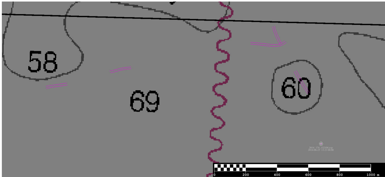
Figure 14: Outer beam refraction errors cause from changing sound velocity throughout the survey area. Data were cleaned thoroughly if outer beam errors exceeded allowable uncertainty values.
