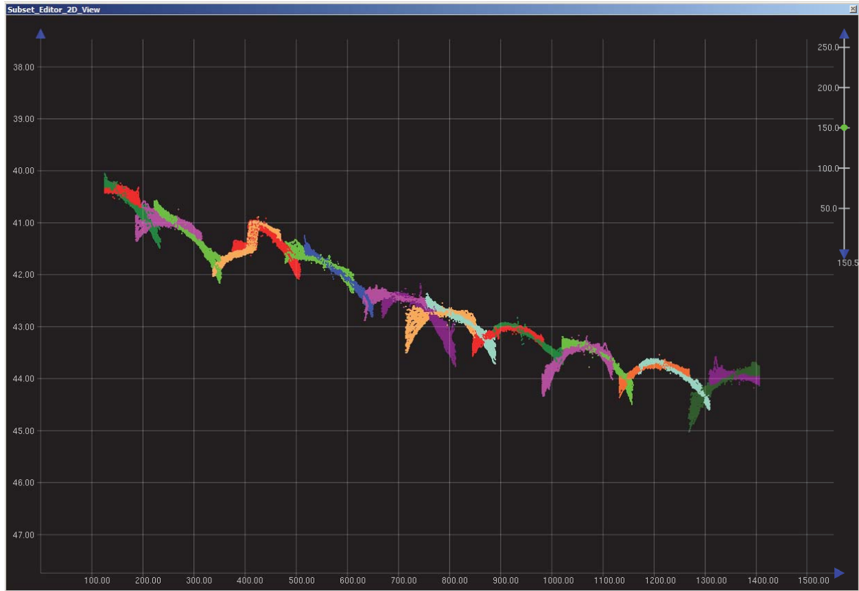
Figure 14: Outer beam refraction errors caused from changing sound velocity throughout the survey area. Data were cleaned thoroughly where outer beam errors exceeded allowable uncertainty values.
