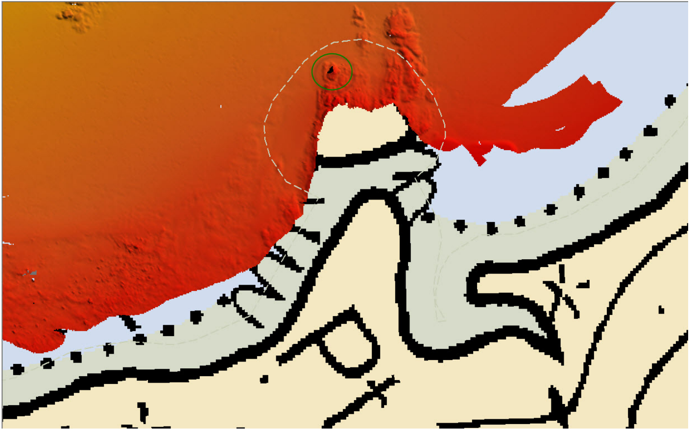
Figure 63: H12741 Graphical Overview of Holiday Due to Steep Downslope of Rocky Coastal Line
