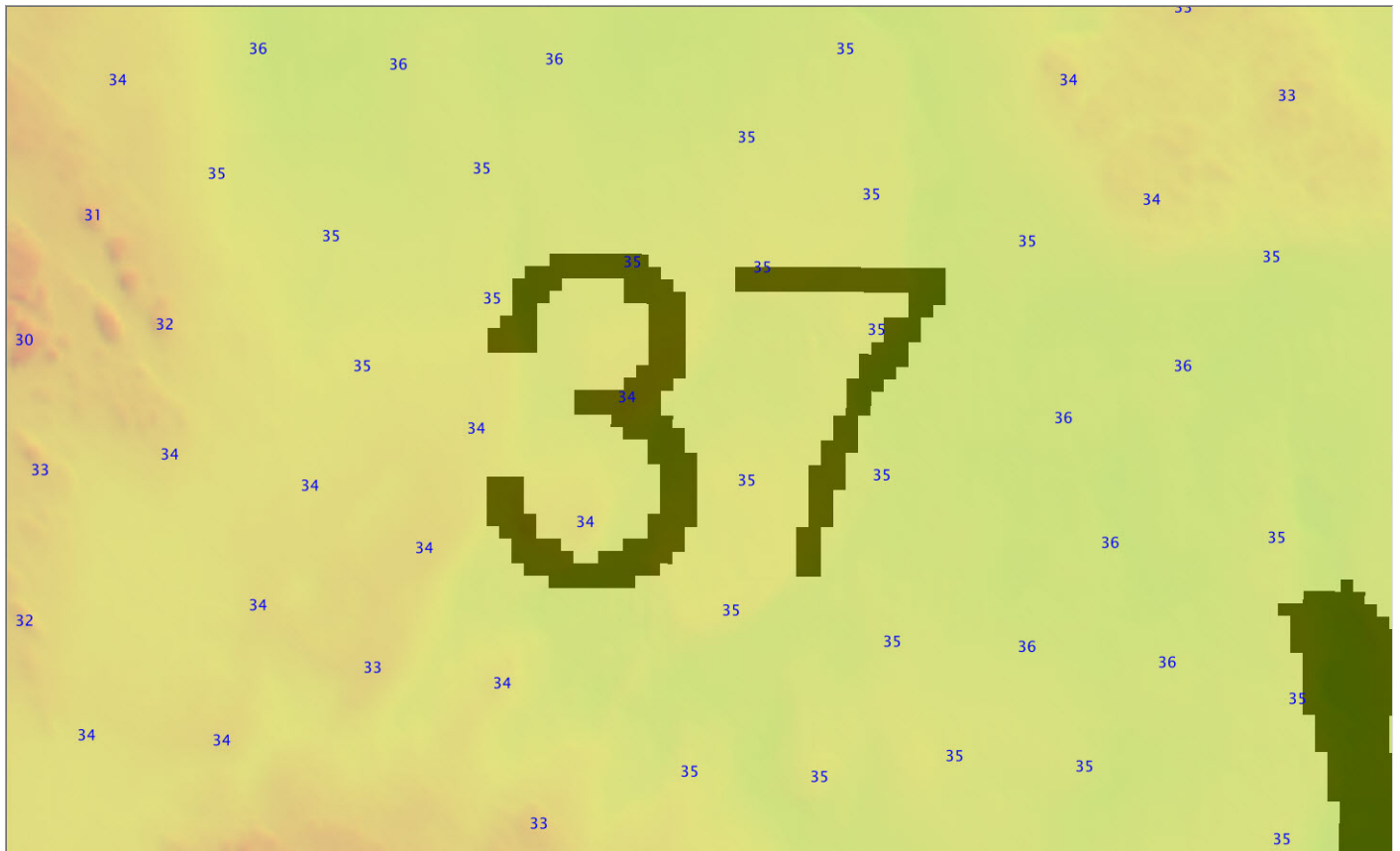
Figure 23: Discrepancy in charted depth vs surveyed depth (2-3 fathoms)
