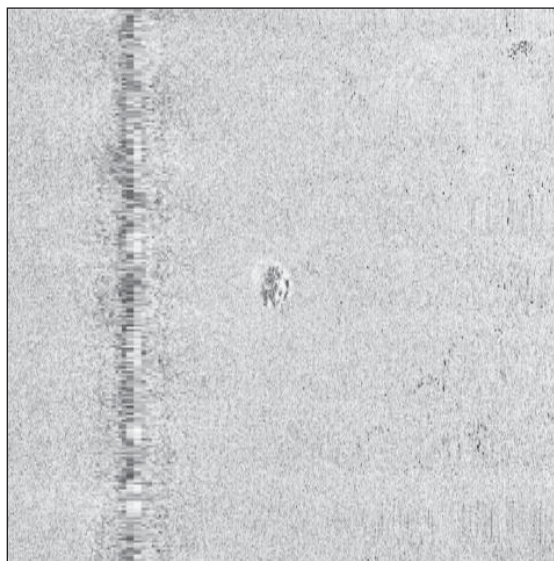
Figure 20. Typical SSS signature of contacts identified along a pipeline within the survey bounds of H12791
