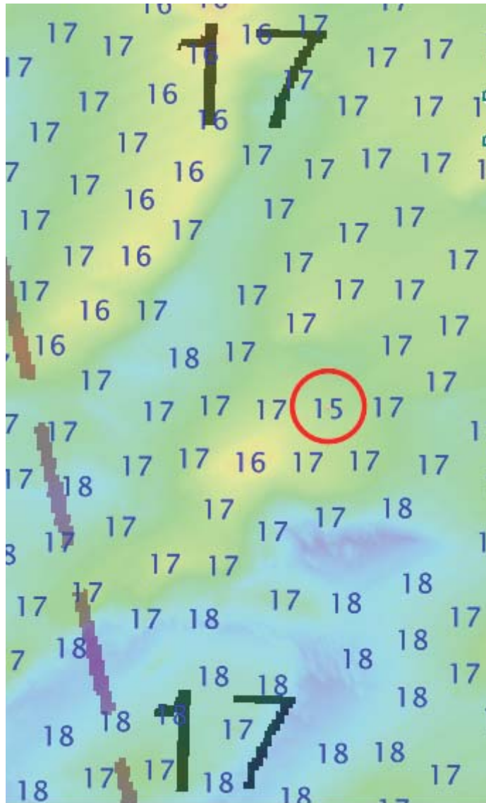
Figure 20: 15 fathom sounding between two charted 17 fathom soundings. General position: 33-16-10 N and 077-57-11 W.
