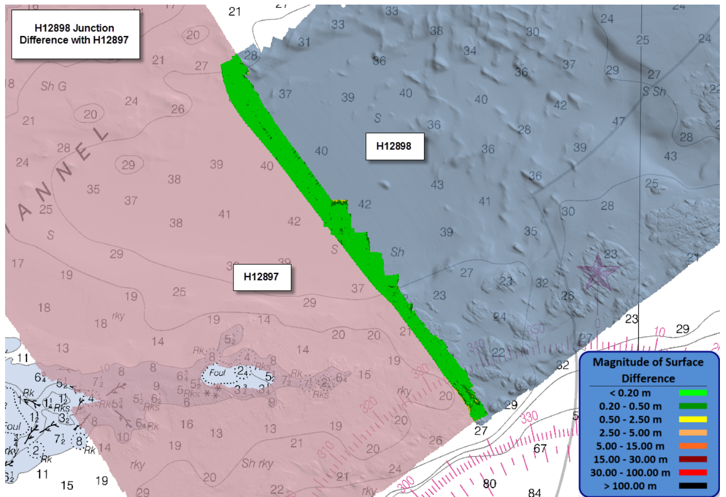
Figure 8: Difference surface between H12898 and junctioning survey H12897.
