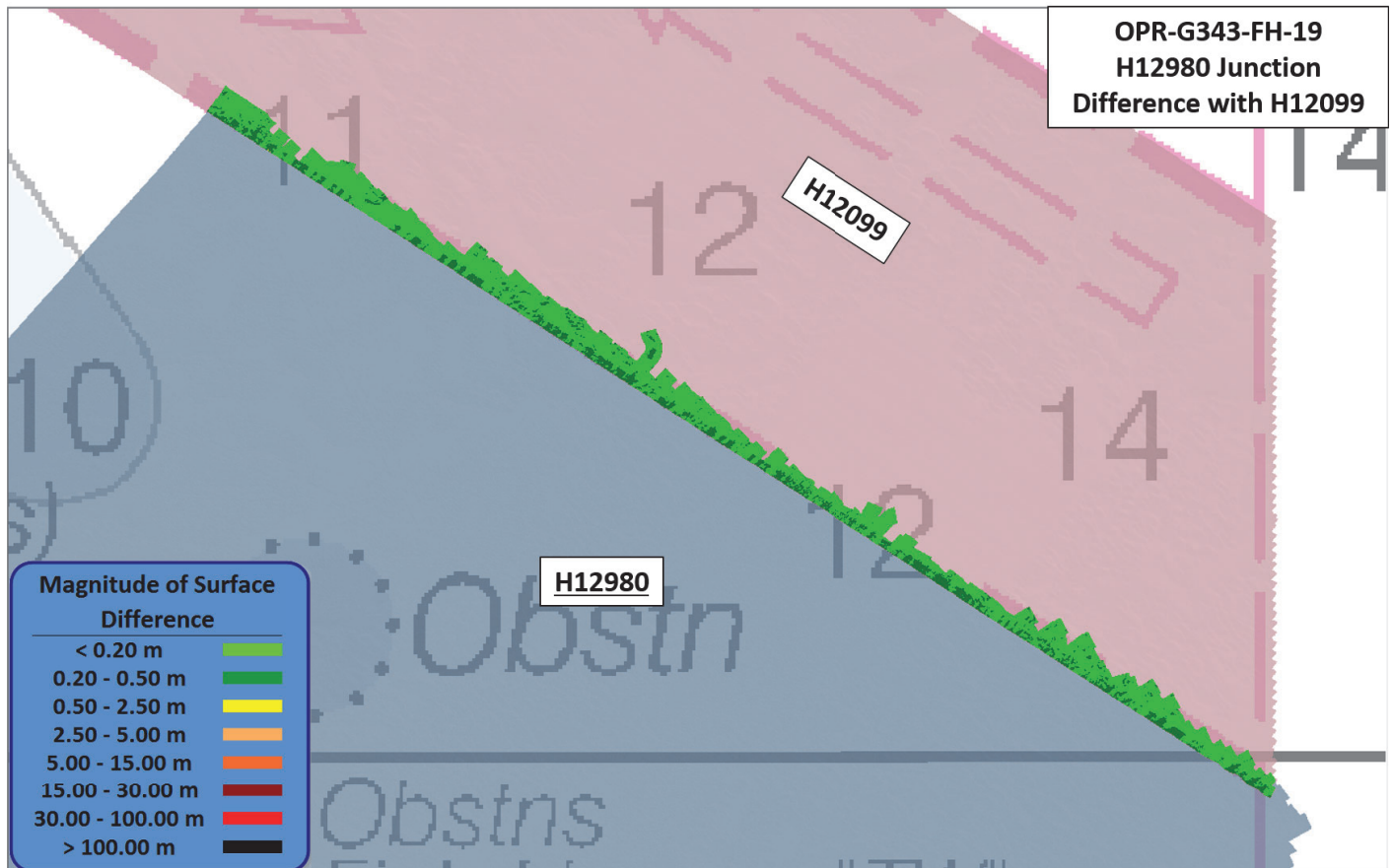
Figure 8: Difference surface between H12980 (blue) and junctioning survey H12099 (pink).
