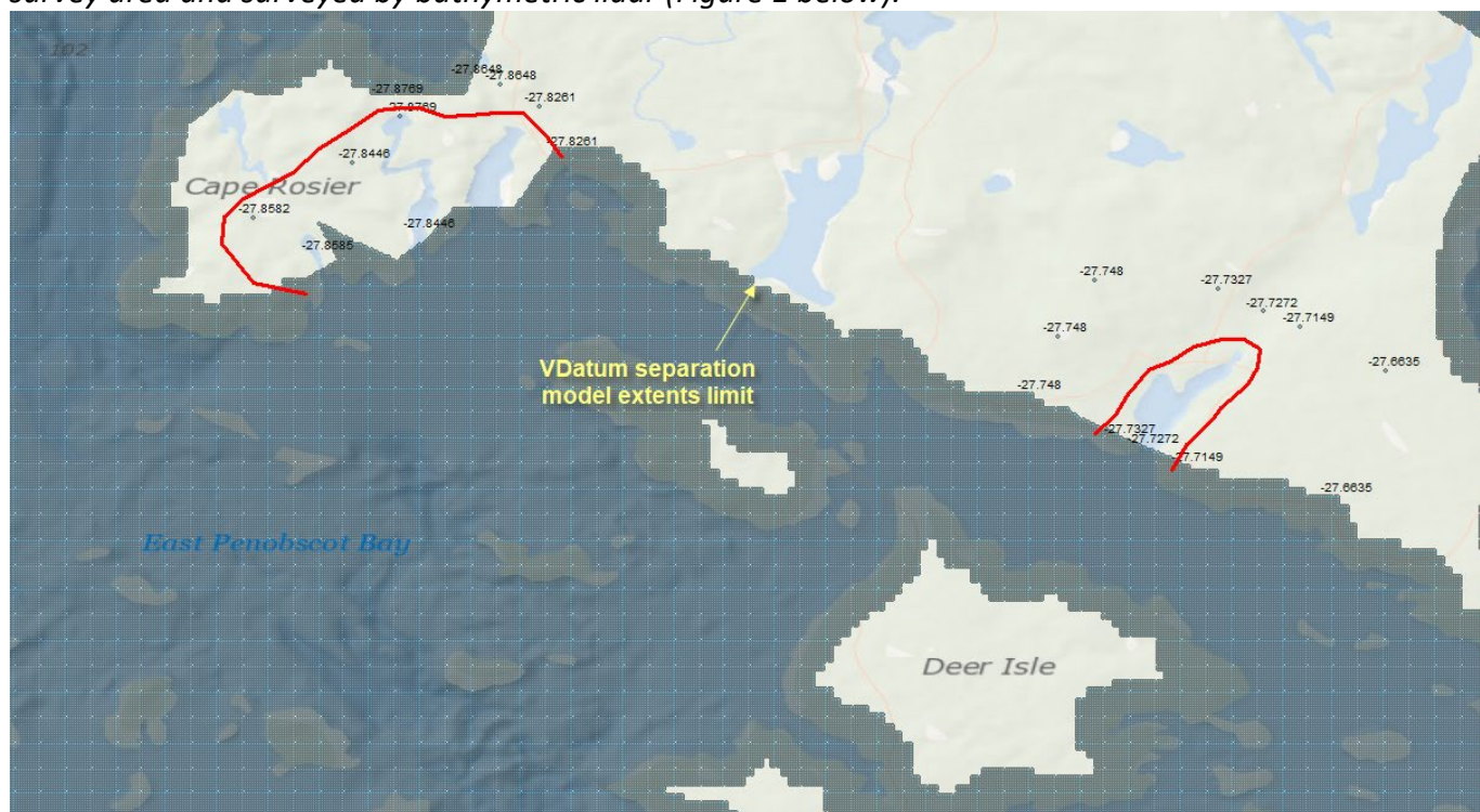
Figure 1. VDatum separation model extents and the areas surveyed by bathymetric lidar not covered by it (in red).
