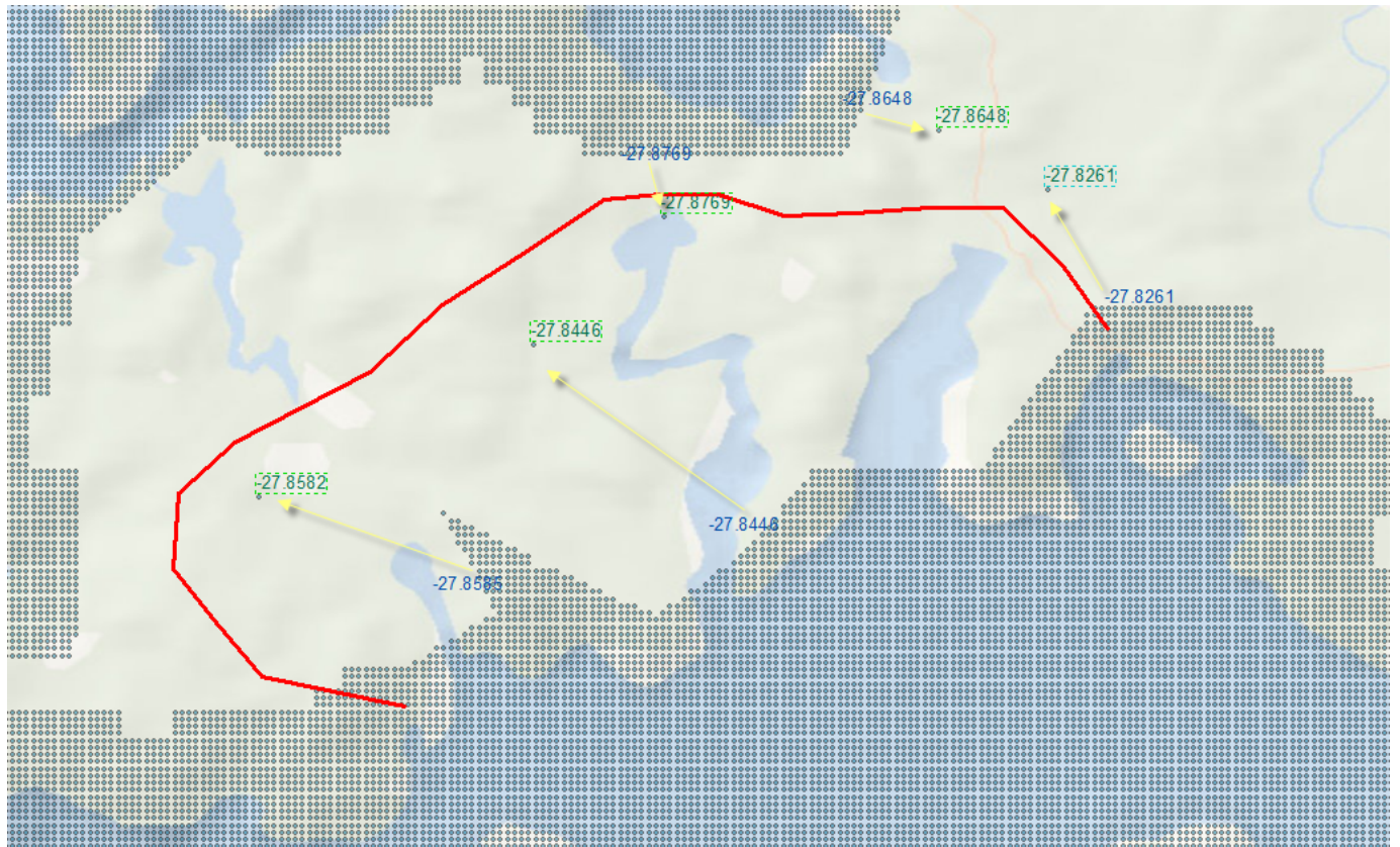
Figure 2. Extrapolation of separation model value at edge limit to include survey area (in red)
