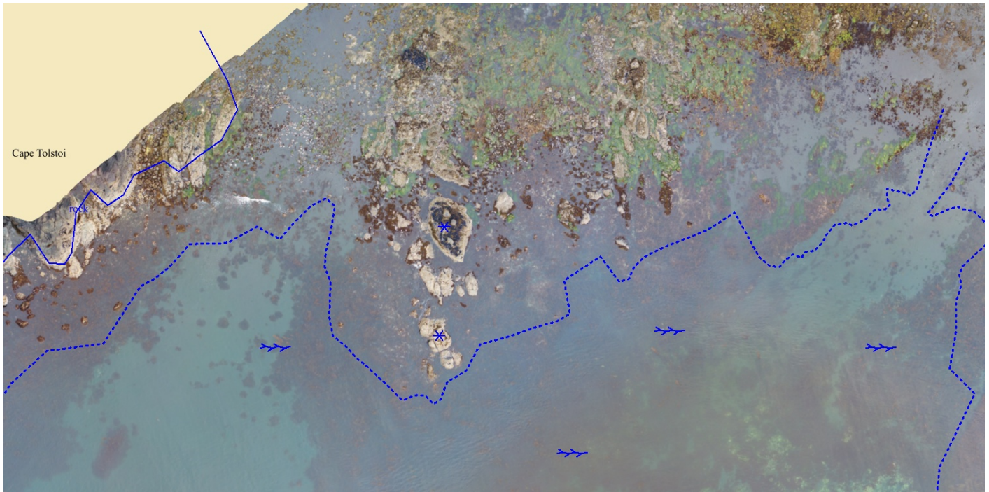
Figure 9: Example orthophotomosaic overlaid with the FFF (blue), showing revised foul limits, ledge lines, rocks, and kelp.
