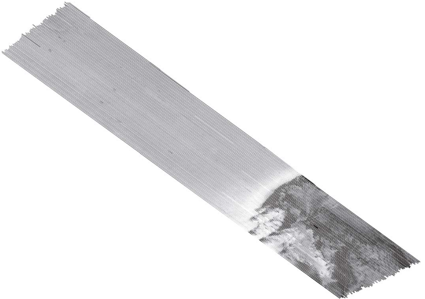
Figure 16: Backscatter GeoTiff processed from data acquired by the Kongsberg EM710 and EM2040.
