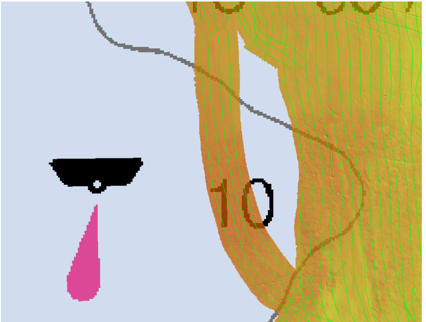
Figure 6: Holiday from surveying around a moored barge
