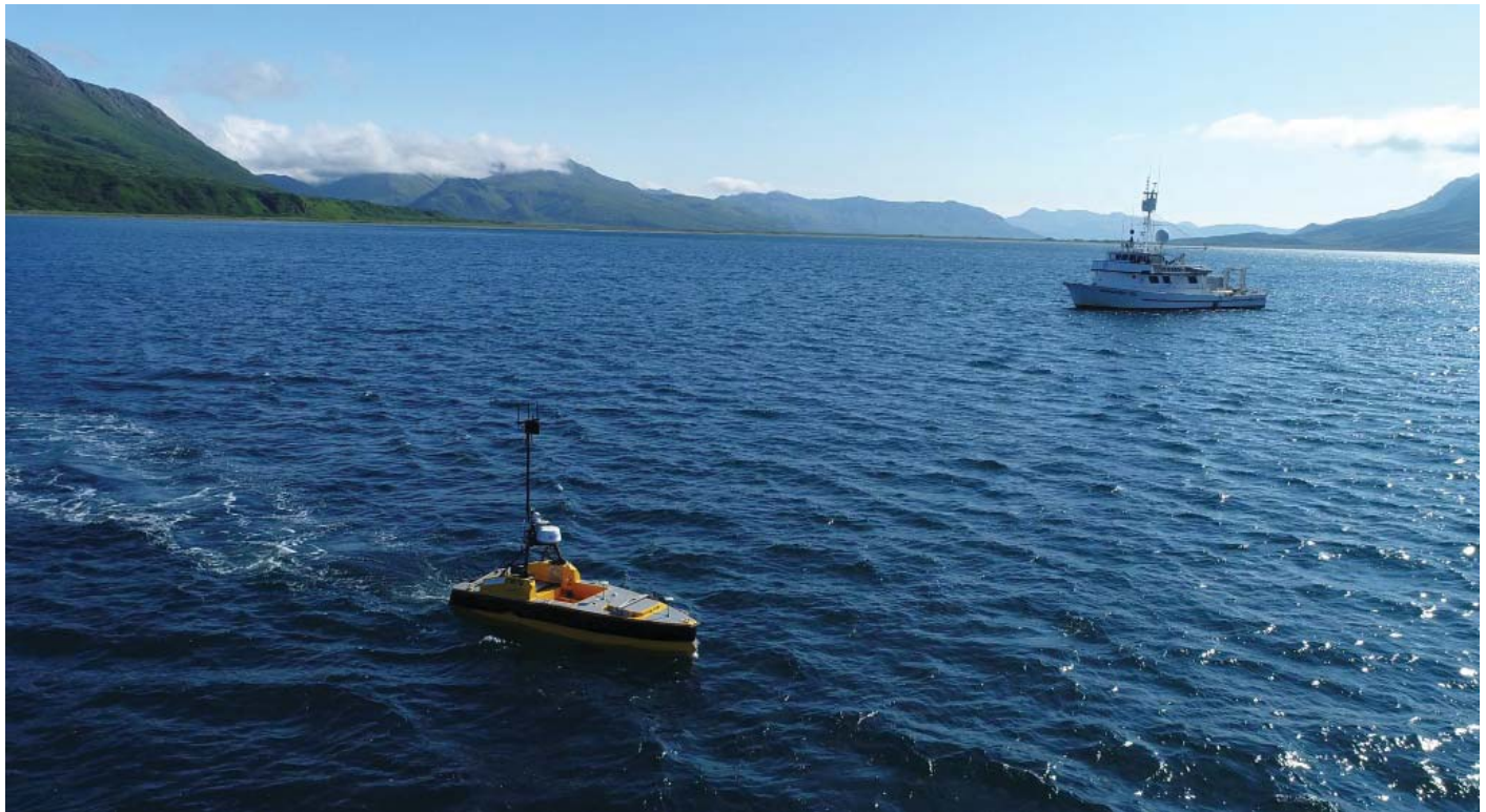
Figure 4: Survey vessels used on this project - ASV-CW5 (foreground), Q105 (background)
