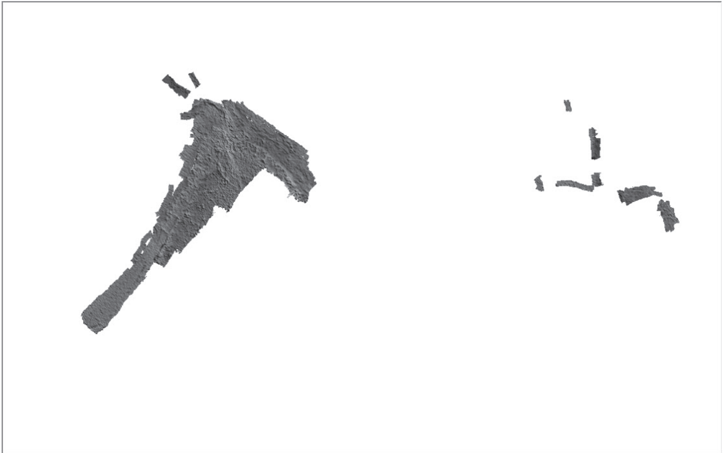
Figure 13: HSL 2903's 200kHz multibeam acoustic backscatter at 1m resolution.
