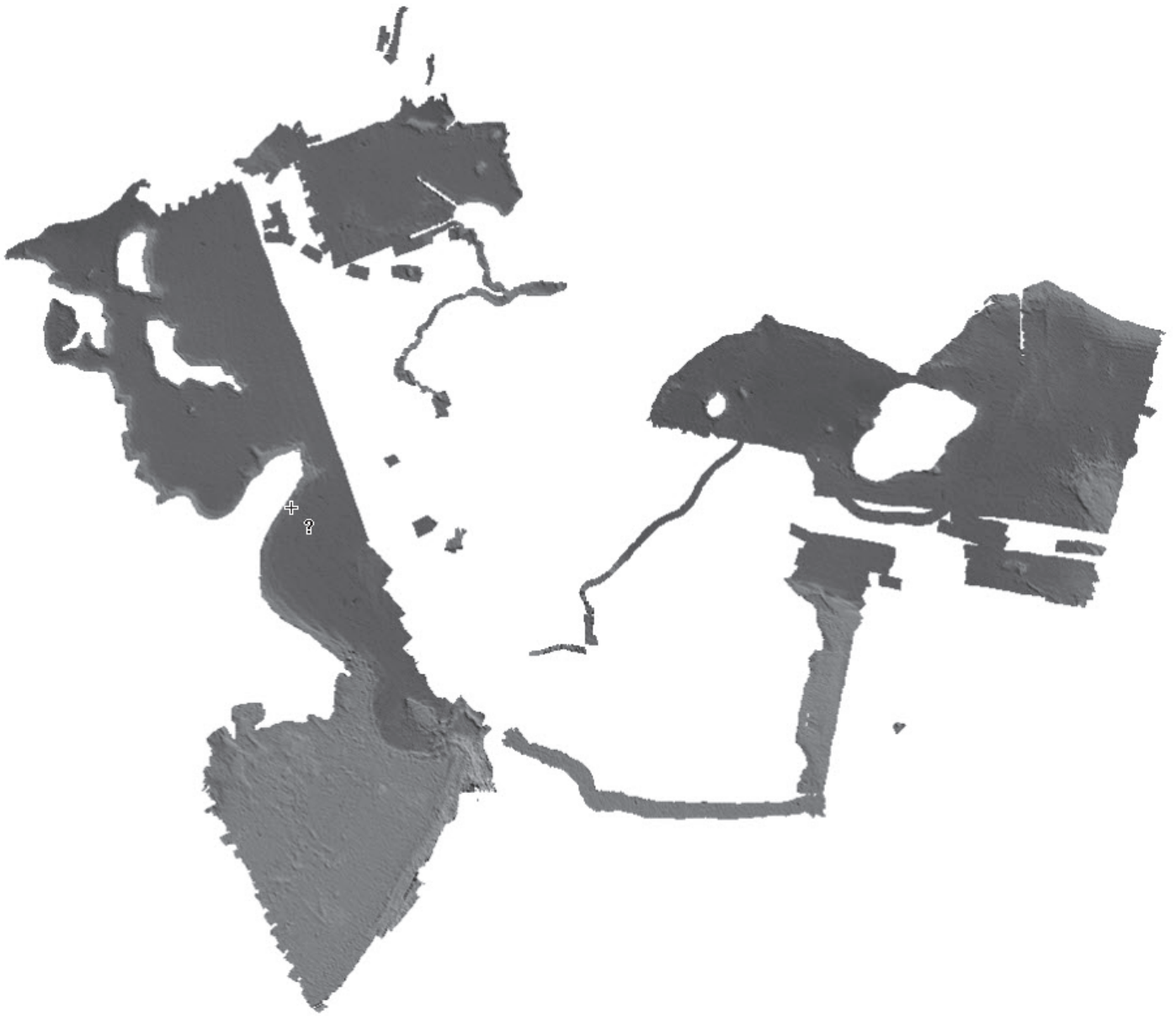
Figure 12: HSL 2903's 300kHz multibeam acoustic backscatter at 1m resolution.
