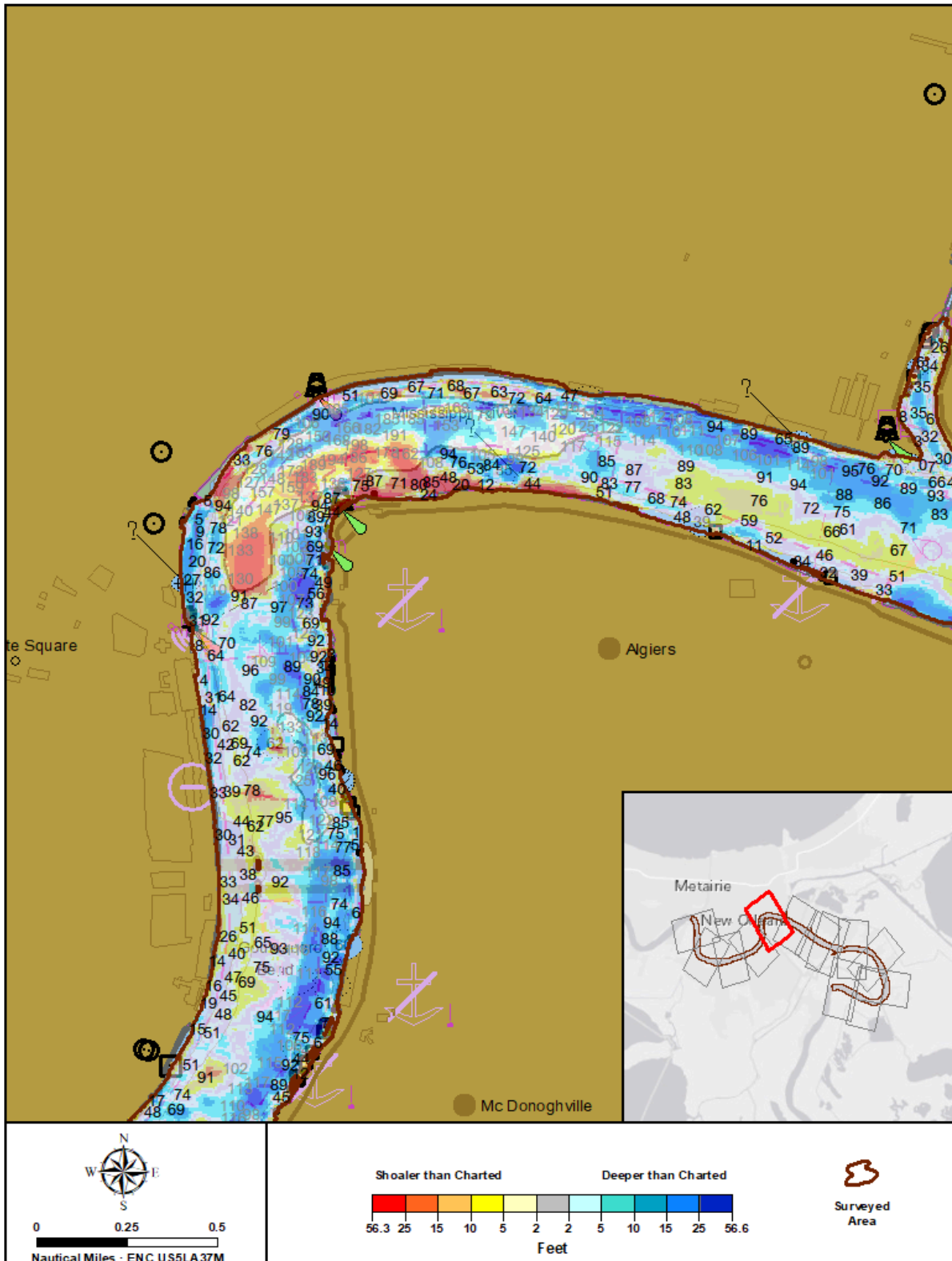
Figure 27: Depth difference between H13193 and chart US5LA37M, area 5 of 7
