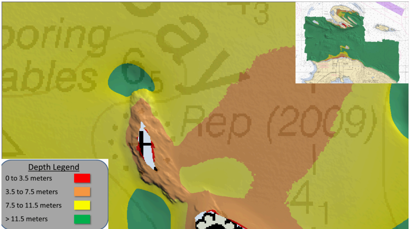
Figure 17: Holiday 6: Reported submerged rock over which a least depth could not be determined
