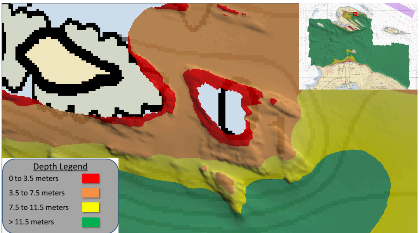
Figure 18: Holiday 7: Charted shoal in Echo Bay that could not be safely developed
