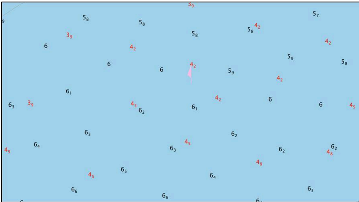
Figure 10: ENC US5TX72M Charted Soundings (red) with H13213 CUBE Depth Selected Soundings (black)
