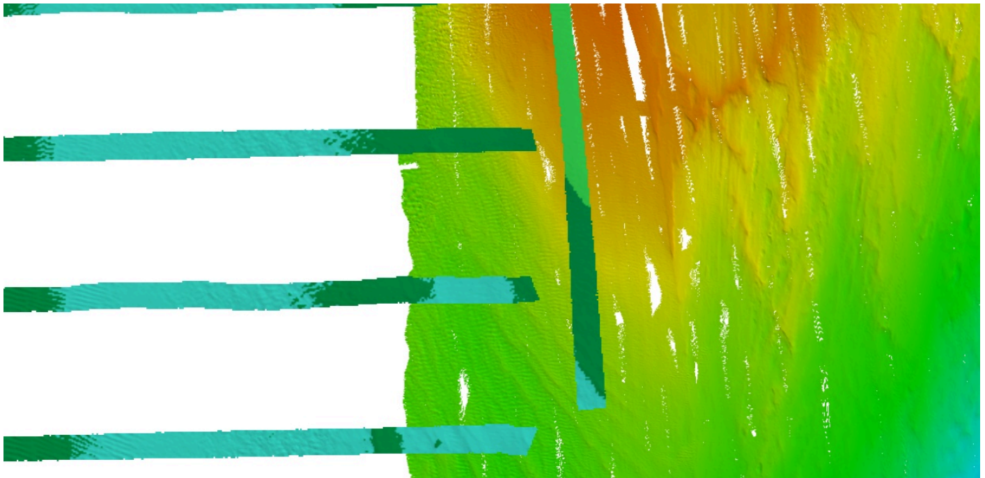
Figure 6: Image showing an area of up to 1 m of disagreement between the 2011 (right side of image) and 2019 (left side of image) surveys. Sandwaves are readily apparent in both data sets.
