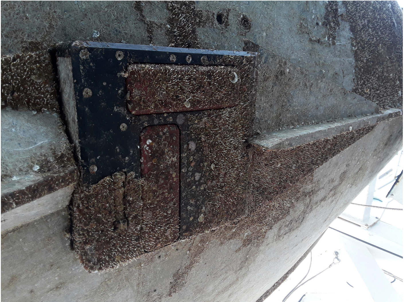
Figure 13: RAINIER launch EM 2040 transducer with biofouling in the process of being cleaned.
