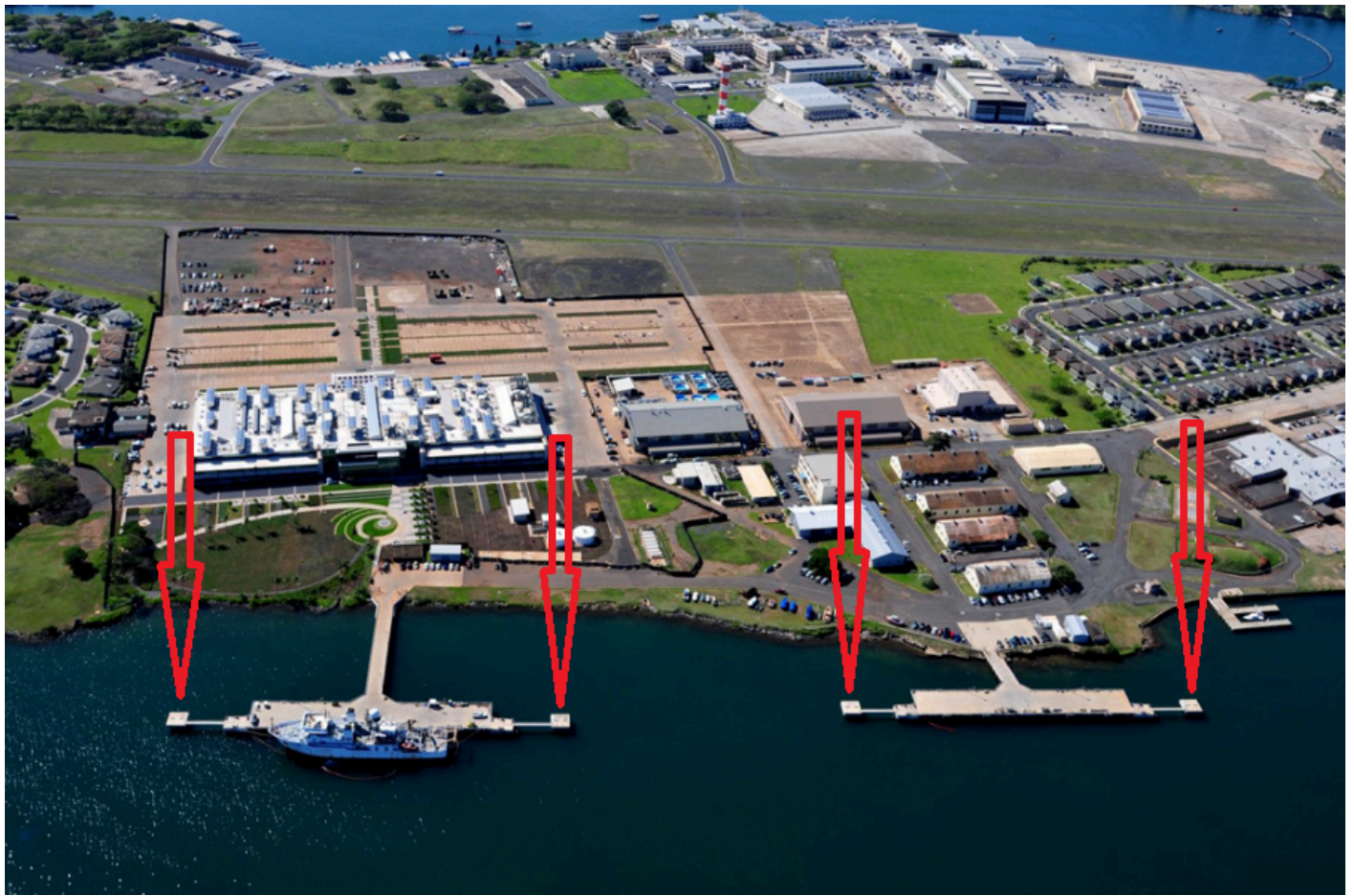
Figure 28: Ship piers at the NOAA Inouye Regional Center with red arrows pointing to four uncharted dolphins with associated catwalks.
