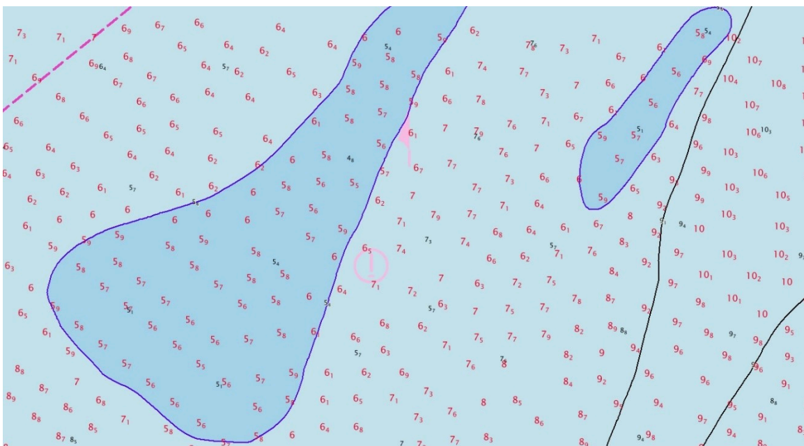
Figure 20: ENC US5VA24M Charted 5.4-meter contour (blue), Charted Soundings (black), H13301 CUBE Depth Selected Soundings (red)
