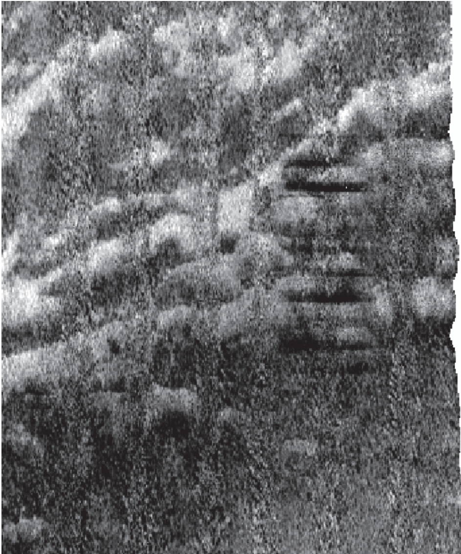
Figure 31: S222's multibeam acoustic backscatter holiday on line 0128_20191028_155009_S222_EM2040 on Julian day number 301. Approximate location of 36° 30' 5.66"N, 75° 22' 9.12"W.
