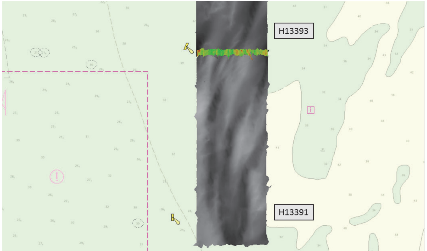
Figure 6: H13393 junctions with the northern edge of H13391.
