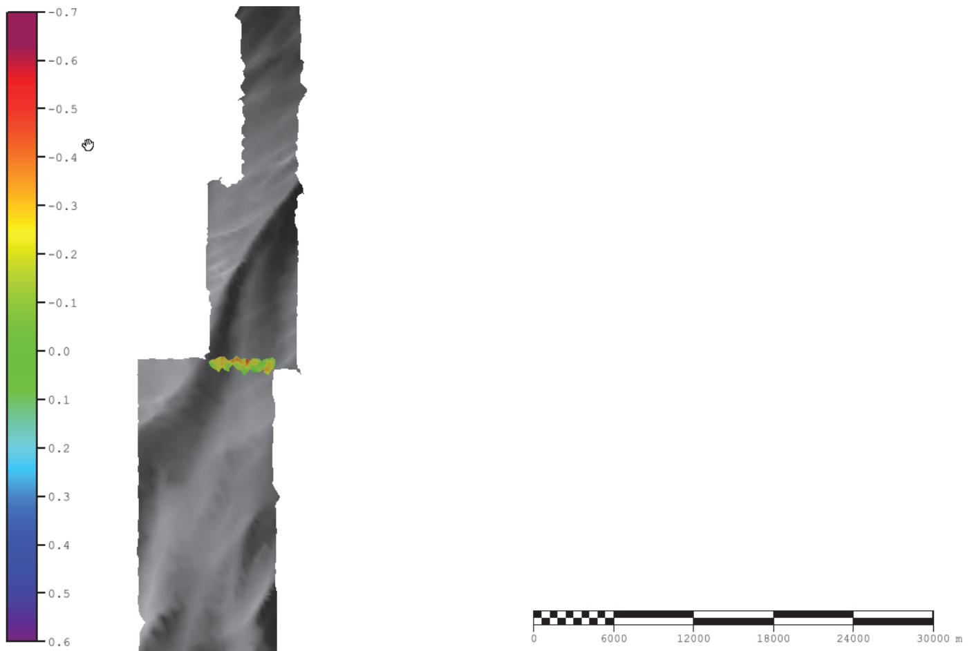
Figure 16: Junction difference surface between Survey H13417 and H13394 in color. Visual inspection indicates that the surveys are in general agreement.
