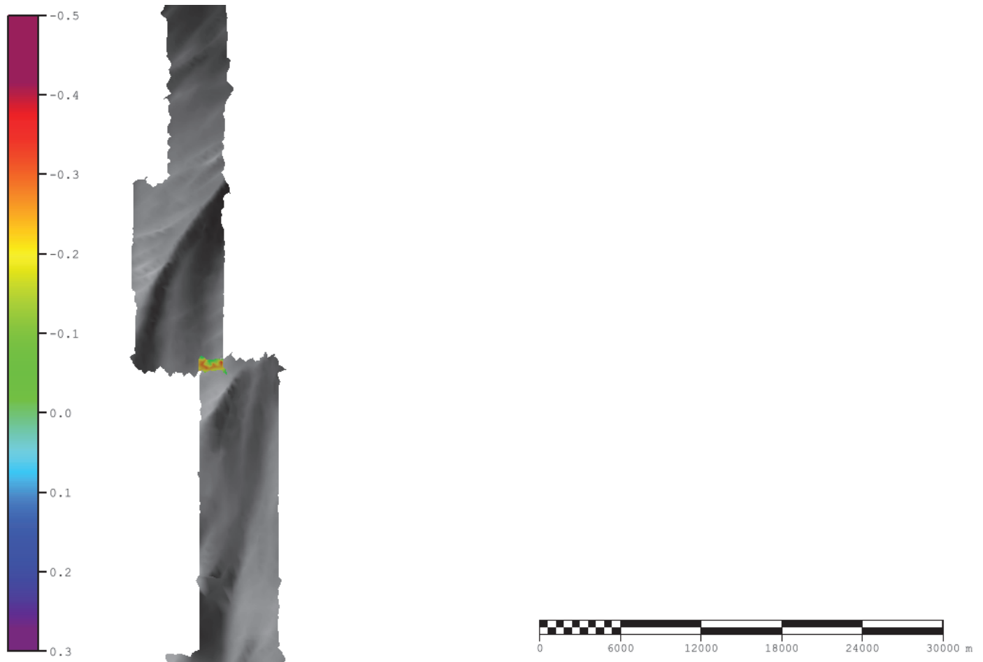
Figure 14: Junction difference surface between Survey H13417 and H13393 in color. Visual inspection indicates that the surveys are in general agreement.
