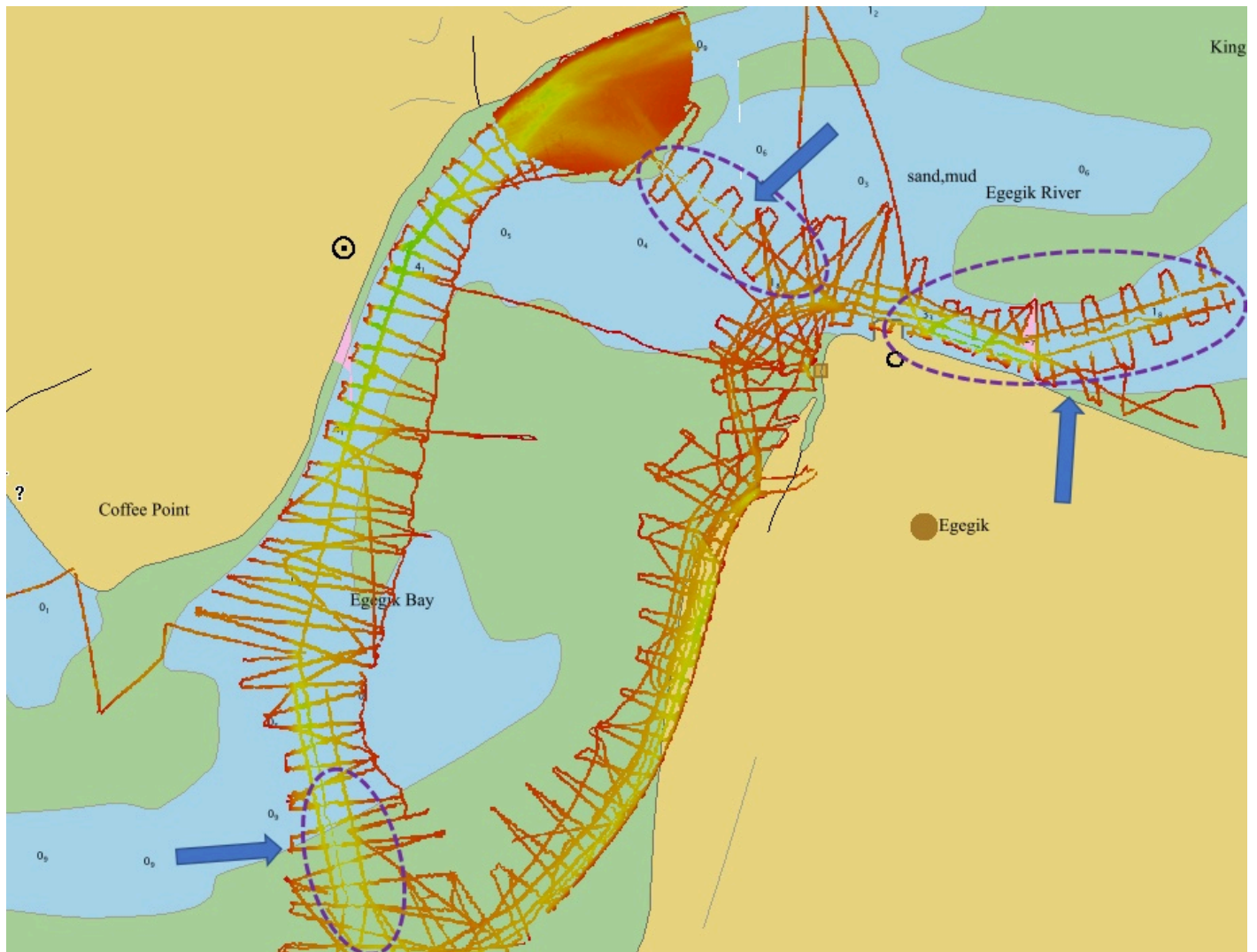
Figure 15: The entire upper river area shown in the diagram was intermittently affected by the bottom tracking issue. However, the areas circled were most affected.
