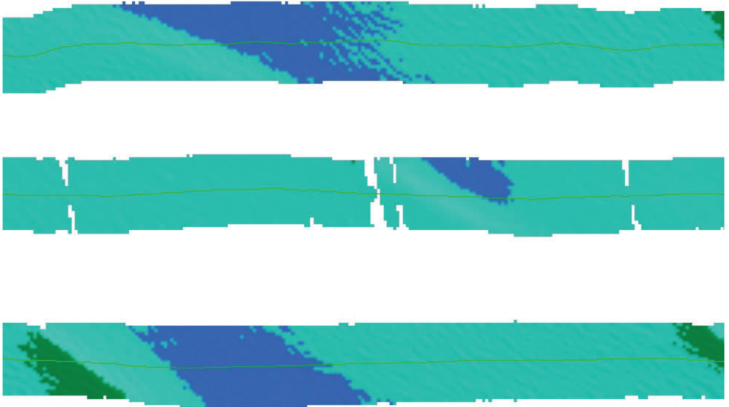
Figure 6: Image of the final surface showing the effect of data blowouts on a line from rough weather.
