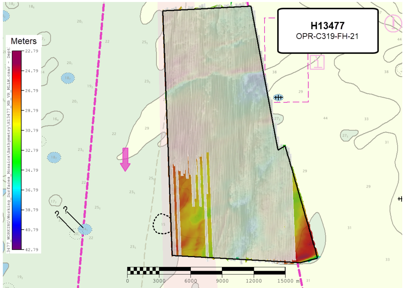
Figure 2: Complete Coverage SSS (greyscale) plotted over MBES coverage acquired on H13477. Black outline represents sheet limits assigned in the PI.
