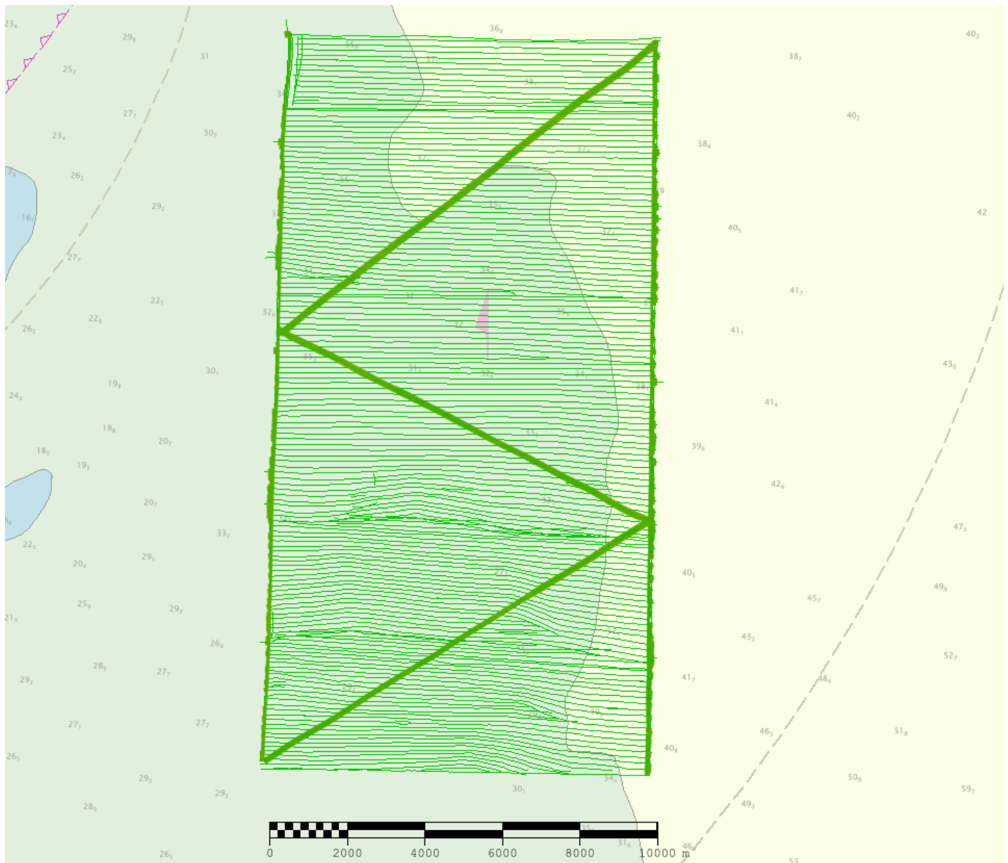
Figure 4: H13594 crossline surface overlaid on mainscheme tracklines. Color scale coded as green = meets IHO standard and red = fails IHO standard (ENC US4NC16M).
