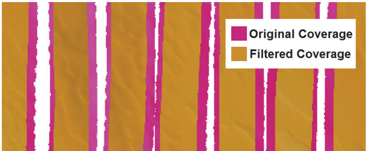
Figure 24: Example of the loss of spatial coverage as a result of filtering the multibeam data logged concurrent with the side scan sonar.
